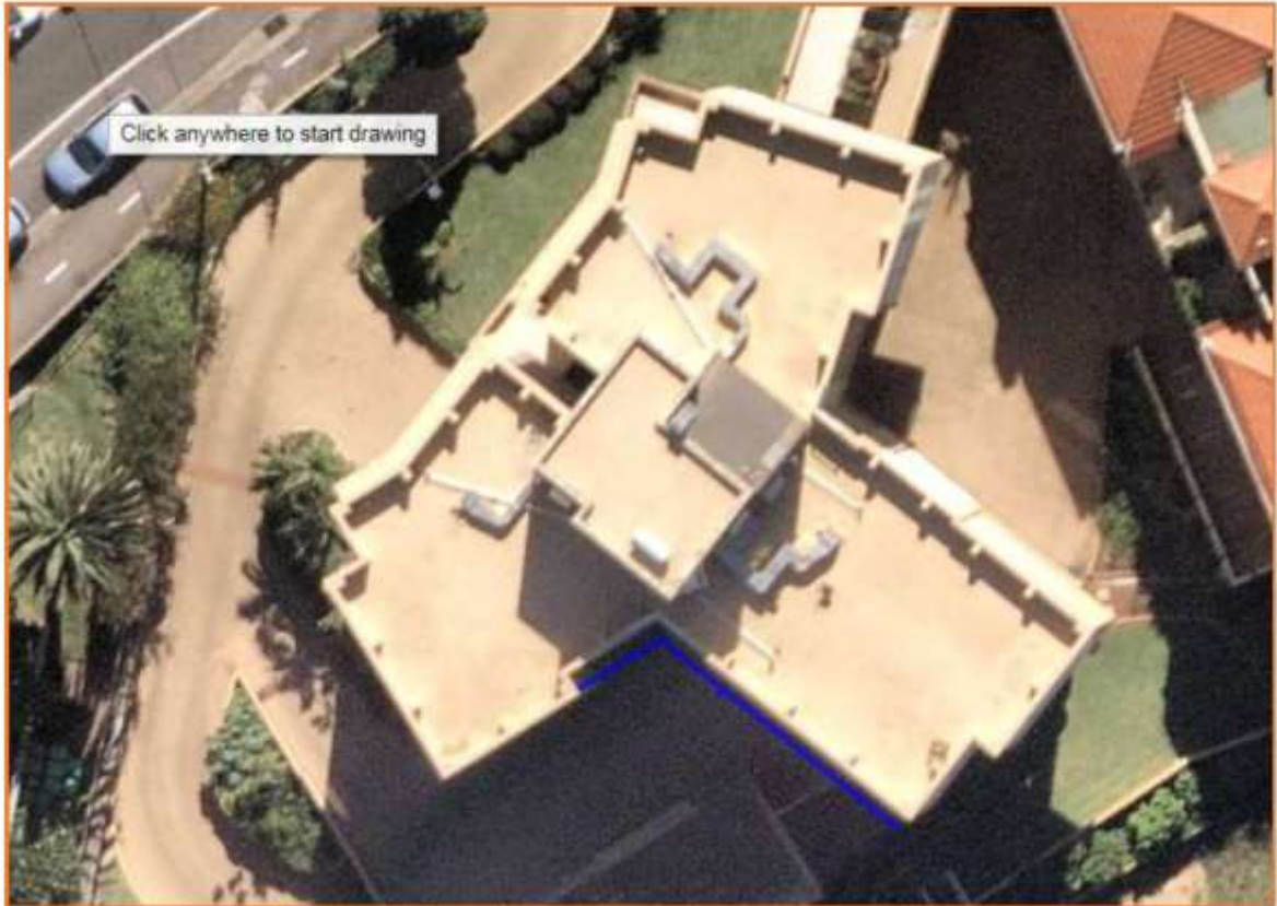
Area marked up in blue for cavity flashing replacement
